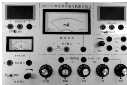
图4 DH4508型电表改装与校准实验仪
