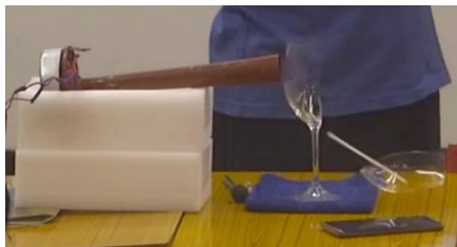
图6 “声音震碎酒杯”实验
